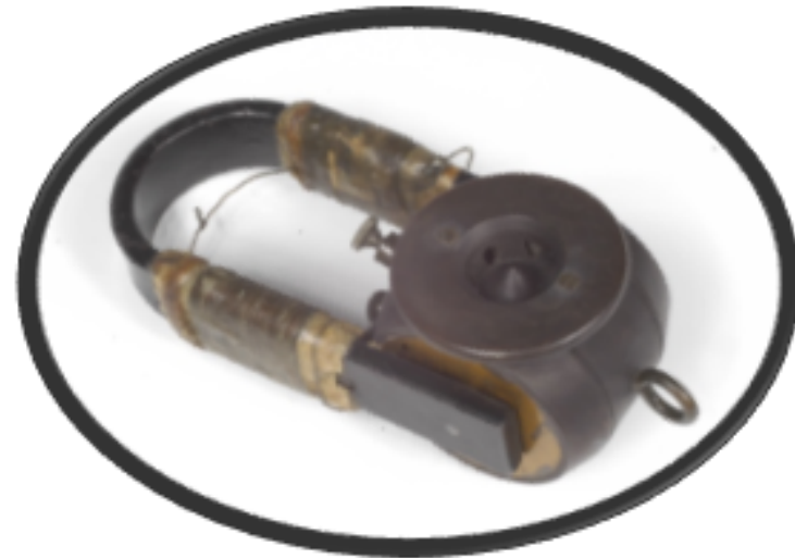
Figure 3 This was held in the hand of the first human being to hear a radio signal sent across the Atlantic - the three Morse-code dots for 'S' - from Cornwall to Newfoundland in 1901
